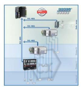
The HART information can also be accessed via the Profibus DP protocol thus allowing for maintenance of the pool of analogue instruments (sensors and actuators).
